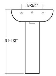
Dimensions of fixture are nominal and may vary within the range of tolerances established by ASME Standard A112.19.2-2018. Dimensions and specifications subject to change without notice.
